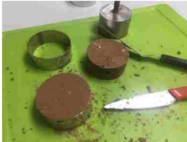
Figure 3-1: Molding of prepared soil samples to be placed in the anaerobic chamber.
