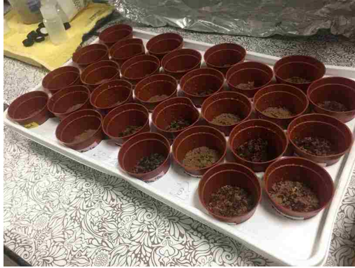
Figure 3-6: The samples for the advanced bioremediation with ZVI being left to incubate. The aluminum foil in the background was prepared to cover the samples and keep them from drying out completely during incubation.
