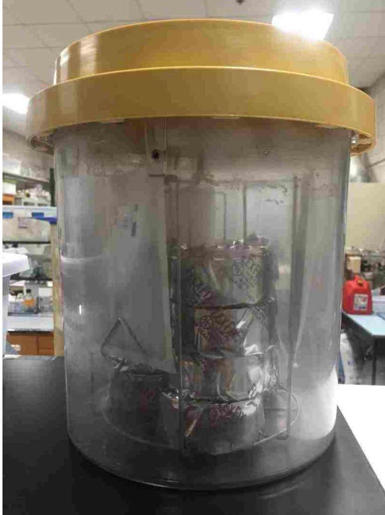
Figure 3-3: Soil samples left in the anaerobic chamber to incubate. More samples were previously in this chamber; the time elapsed for the experiment at the time this picture was taken was at least 35 days.
