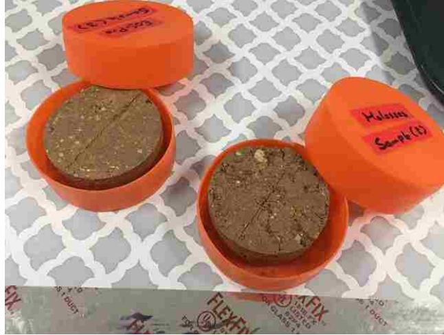
Figure 3-2: Finished soil samples placed in labelled Shelby tube end caps. These were wrapped in aluminum tape to prevent any air from reaching the samples, effectively sealing them completely. The lines in each sample indicate how much to take for contaminant analysis.
